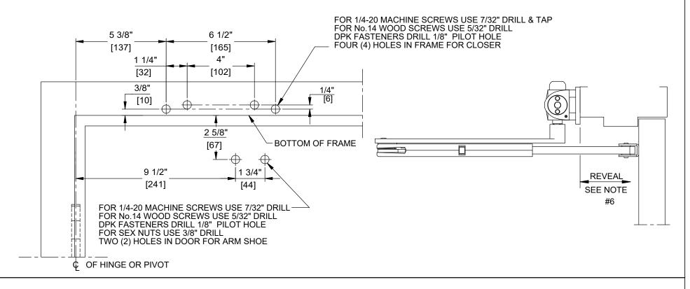
DOOR CLOSER MODELS: 8616 PHJ TOP JAMB INSTALLATION (PUSH SIDE MOUNT) PLUNGER HOLD OPEN ARM WITH PLATES BP86, BP86FC
