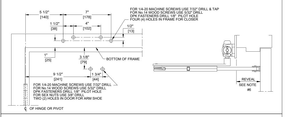
DOOR CLOSER MODELS: 8616 PHJ TOP JAMB INSTALLATION (PUSH SIDE MOUNT) PLUNGER HOLD OPEN ARM WITH PLATE DP86
