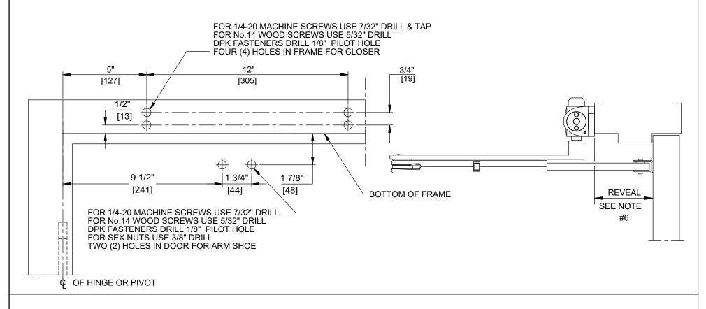
DOOR CLOSER MODELS: 8616 PHJ TOP JAMB INSTALLATION (PUSH SIDE MOUNT) PLUNGER HOLD OPEN ARM
